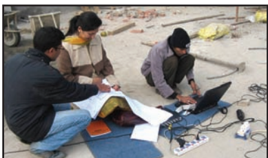
Microtremor Equipment during field visit in Building assessment
